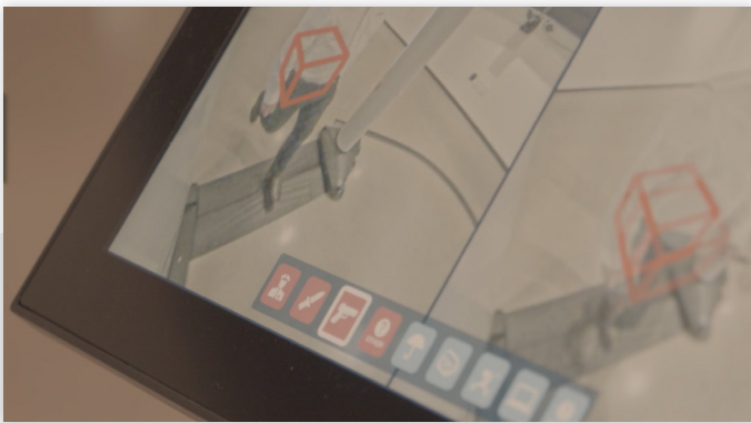
When an operator at the Evolv Express system tags a threat item on the tablet (above, left), the threat localization image and alert metadata (time, location, and threat type) are sent to Genetec (below, upper LH quadrant). Requests for assistance (above, right) made from the tablet are also displayed in the Genetec user experience, and they may be communicated with or without an accompanying verified alert.
